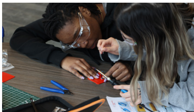
Figure 1. Students practice soldering a 3D printed low-profile adaptive switch in the Makers Making Change workshop.
